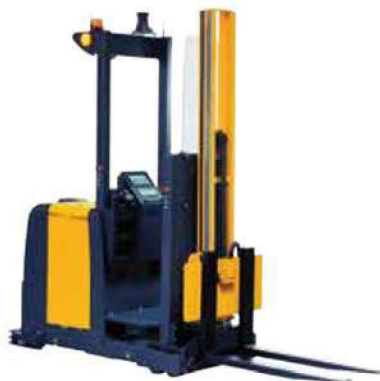
FIE 118 Electric Reach Stacker Cap: 500 /1000/1500 kgs Max lifting ht: 15 Mtr.
