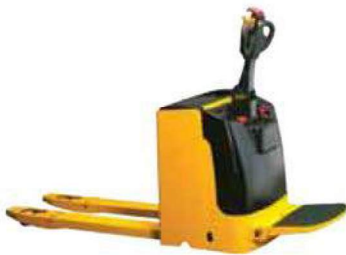
FIE 108 Battery Operated Pallet Truck Cap: 2200 kgs
